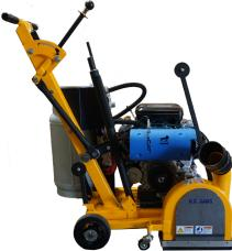
U.S.SAWS JS-160P is a Joint Clean-out Saw/Mill designed to cleanout existing control joints to prepare for new joint fill application or to remove failing or deteriorated existing joint fill material. This machine can be used to remove polyurea, epoxy, and polyurethane joint fill materials. This JS-160P has several key features to provide accuracy, high production rates, and a safe working environment.
